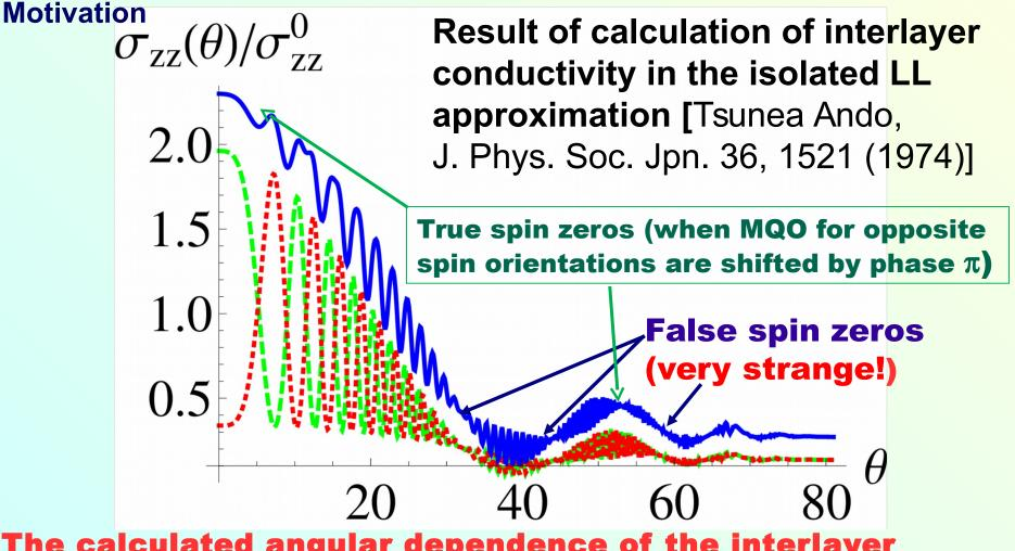
The calculated angular dependence of the interlayer conductivity for spin-up component ( dashed green line), spin-down component (dotted red line), and the their sum (solid blue line) for the g-factor g=2 for Gaussian LL shape. Expected false spin-zeroes at angle θ ≈ 32°, 44°, 58°, ... Incorrect, as will be shown later!
