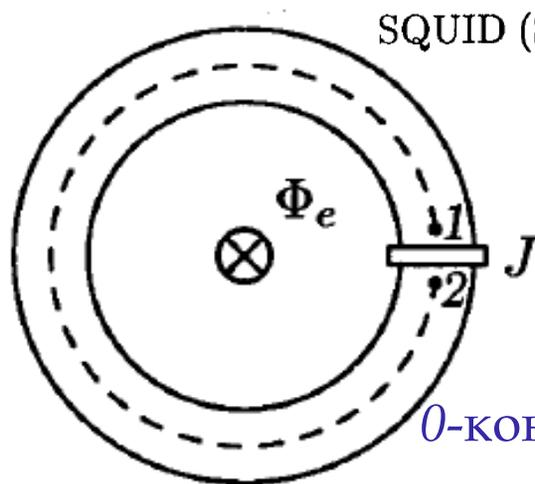
SQUID (Superconducting Quantum Interference Device)
